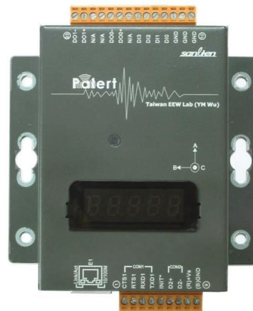
The Palert Earthquake Early Warning (EEW) Unit
